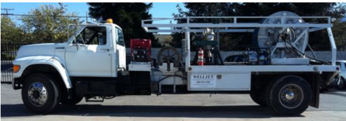
Reel truck – dispenses custom-built high-pressure hose in 1,800' lengths
