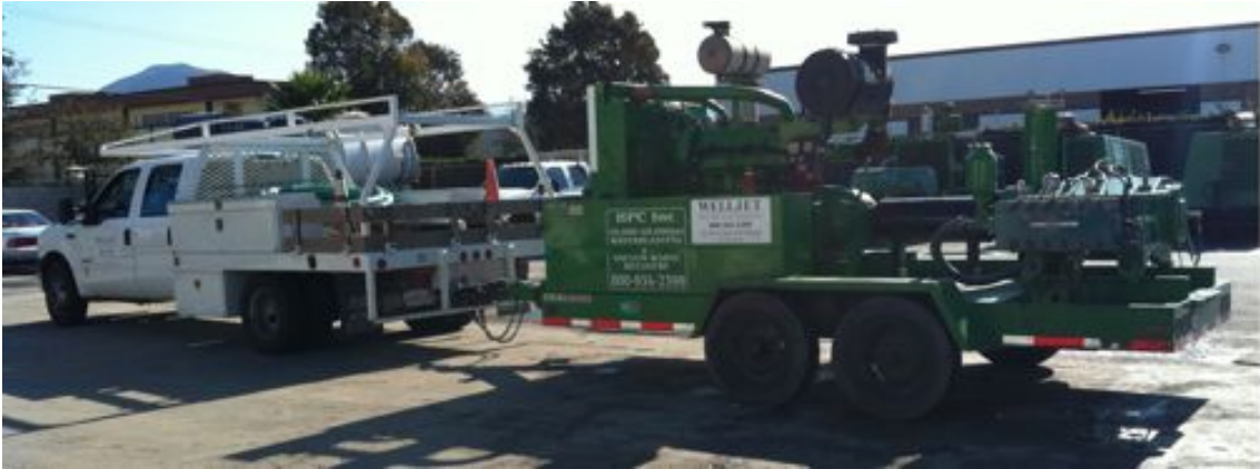
Pump truck – 500 hp diesel generates up to 20,000 psi
